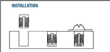
To install, simply press the insert into the hole. The insert compresses as it is installed. As the fastener is threaded into place, the insert expands and the diamond knurling secures it in place.
