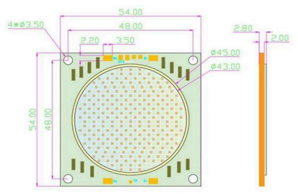
Unit: mm All unmarked tolerances are: +-0.2mm Base plate material: copper substrate
