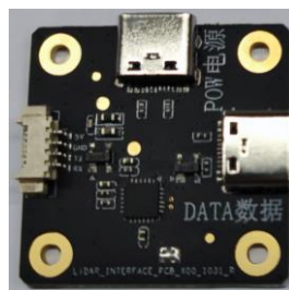
Figure 6-2 Oradar MS200k power adapter board
