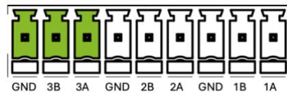
The reComputer R1000 is equipped with 3 sets of RS485 interface using 3-pin connector, which is isolated for both signal and power to ensure safe and reliable operation in industrial and automation applications. The RS485A and RS485B signals are isolated using capacitive isolation, which provides excellent EMI immunity and meets the high-speed communication requirements of the RS485 interface.
