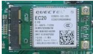
Figure 638: mini-PCIe Connector & 4G Module
