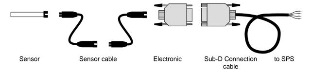
Variant 2: Connection using DIN rail adapter
