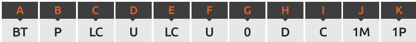
**Example:** BTPLCULCU0DC1M1P = Beyondtech | Patch Cables | LC | UPC | to LC | UPC | OS1 | Duplex | 3.0mm PVC | 1Meter | 1 Pack
