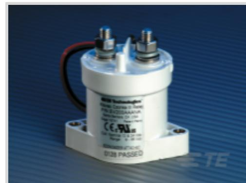
Contact Voltage Rating: **12 - 900 VDC**Contact Arrangement: **1 Form X, SPST-NO**Coil Termination Connection Type: **Flying Lead**High Voltage Connection (Power): **Terminals**Power Switching: **Yes**
