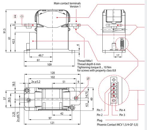
• C300-500-R0P-xxI-V1: Version with PWM module, for top-hat rail mounting
