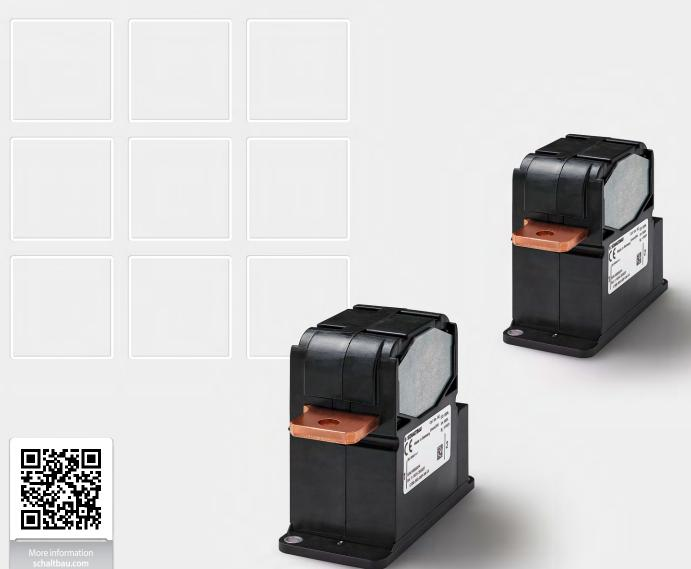
Compact single-pole NO contactors for AC and DC up to 1,500 volts rated insulation voltage. Making current up to 6,000 amps; conventional thermal current up to 500 amps; short-time current up to 6,000 amps.
