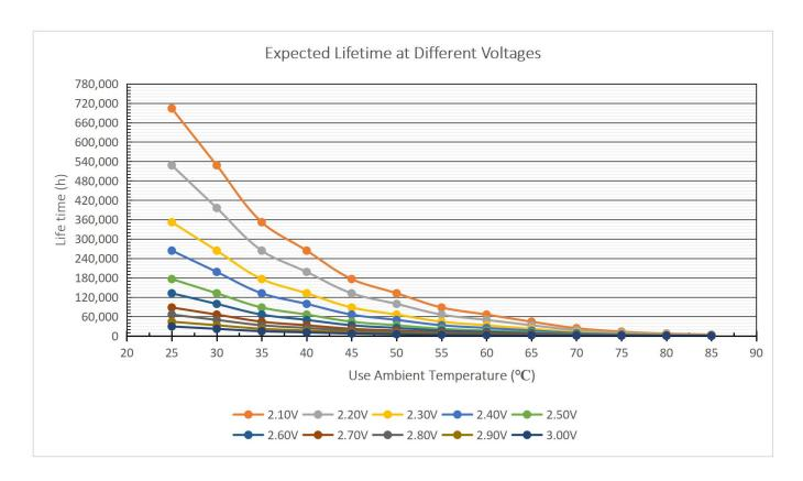
\*Note: Estimated lifespan: The estimated lifespan under different operating voltages and operating temperatures in a theoretical environment. For the actual service life, please contact us to discuss the working conditions.
