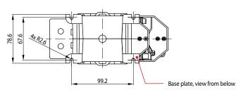
The contactors are mounted on a suitable mounting plate with four M5 screws.
