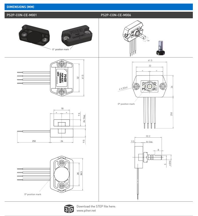
Magnet shown on 0° position. Drawings may not be to scale. Number and function of wires pictured in this datasheet may vary according to output configuration.
