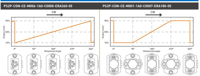
Custom output functions with up to 4 programmable points on request.
