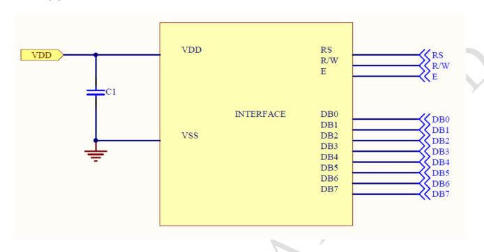
Pin connected to MCU interface: RS, R/W, E, DB0~7
