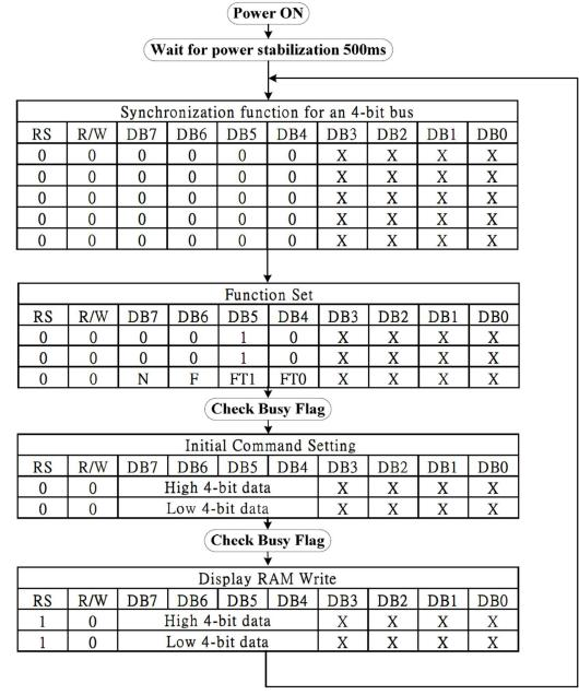
Note: Initial code is for reference only. Please make the best adjustment with the OLED module.
