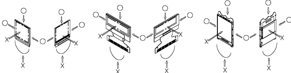
(9) Do not apply stress to the LSI chips and the surrounding molded sections.
