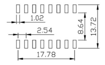
$\label{eq:Suggested} Suggested \ pad \ layout$  Dimensions are in millimeters with the following tolerances: X.XX =  $\pm 0.10$
