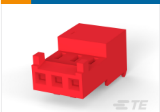
TE Part # 4-643813-6 Nylon Tin Plated Receptacle: 2.54 mm, with Mating Alignment, MTA 100
