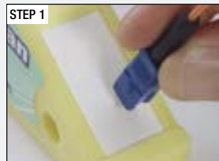
Softly press fiber tip in cleaning window using a figure 8 motion.
