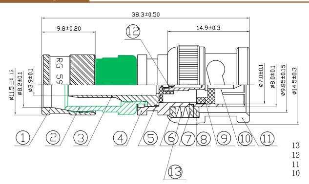
Material Brass Plating Nickel Plastic bush DuPont Delrin 527UV\* Dimensions (height x diameter) mm 27x5.5 Weight kg 0.015
