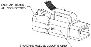
2 POS, PLUG, SOCKET, ATM SERIES, SNAP FIT
