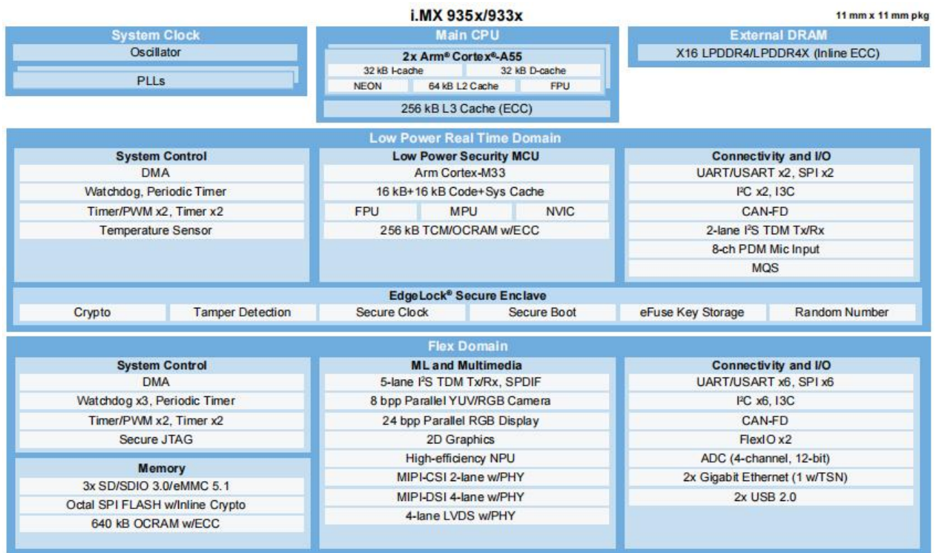
i.MX93 Processor Block Diagram
