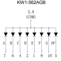
Internal Circuit Diagram (Common Cathode)
