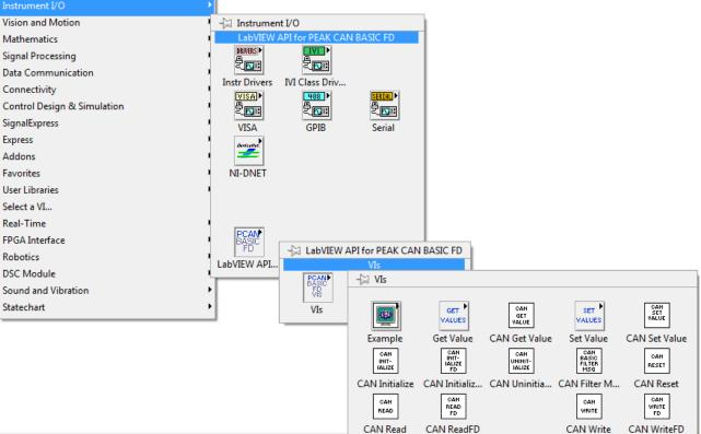
Get and Set Value VIs are accumulated in the VIs CAN Get Value.vi and CAN Set Value.vi. Both VIs are polymorphic to make programming comfortable.
