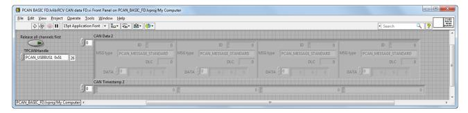
The front panel shows the TPCANHandle (channel) and two arrays for messages and timestamps.
