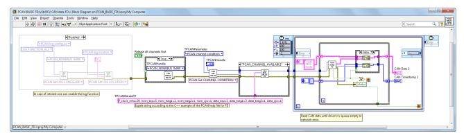
The disabled code segment is followed by the initialisation of the TPCANHandle (channel) and the hardware initialisation. Here is the biggest difference between CAN 2.0B and FD. FD is initialised by a string and not by API VIs.
