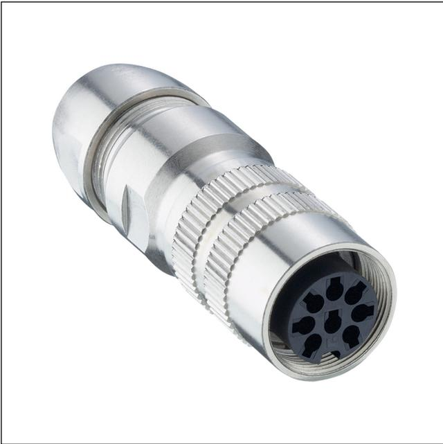
Next Generation – socket acc. to AISG specification and IEC 61076-2-106, IP68, with threaded joint and vibration protection, empty housing for reception of crimp contacts, 360° shielded, optimized assembly
