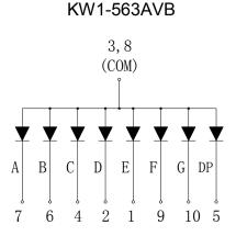
Internal Circuit Diagram (Common Cathode)
