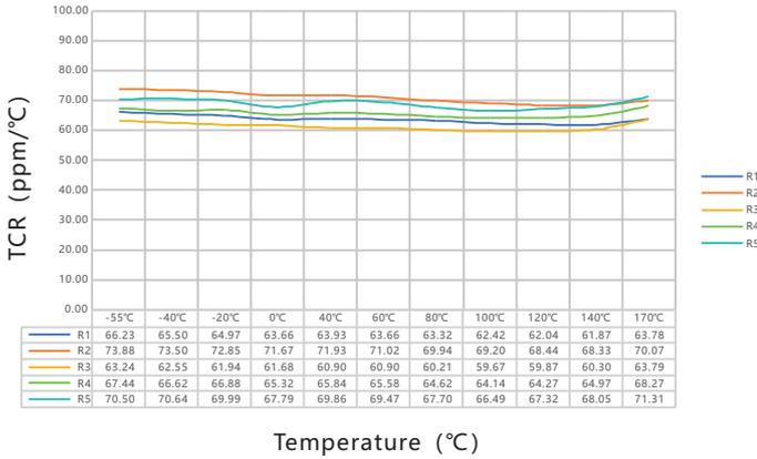
TCR Test Curve -EBWK2512 3mΩ
