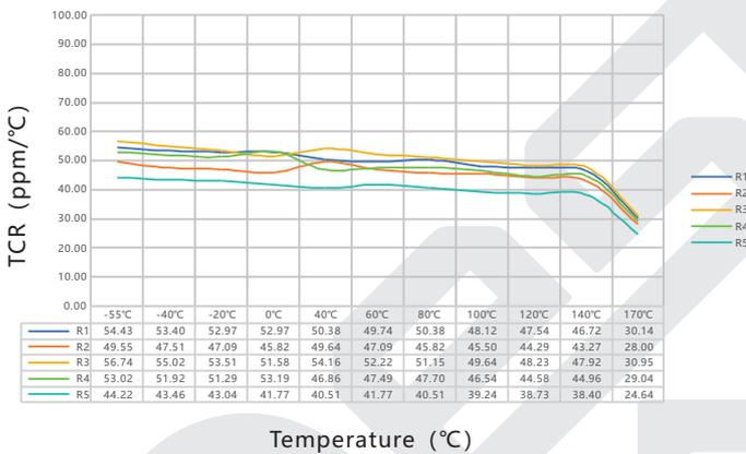
TCR Test Curve -EBWK2512 5mΩ
