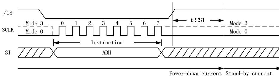
**Figure 7.3.2b.** Release Power-down / Device ID Instruction
