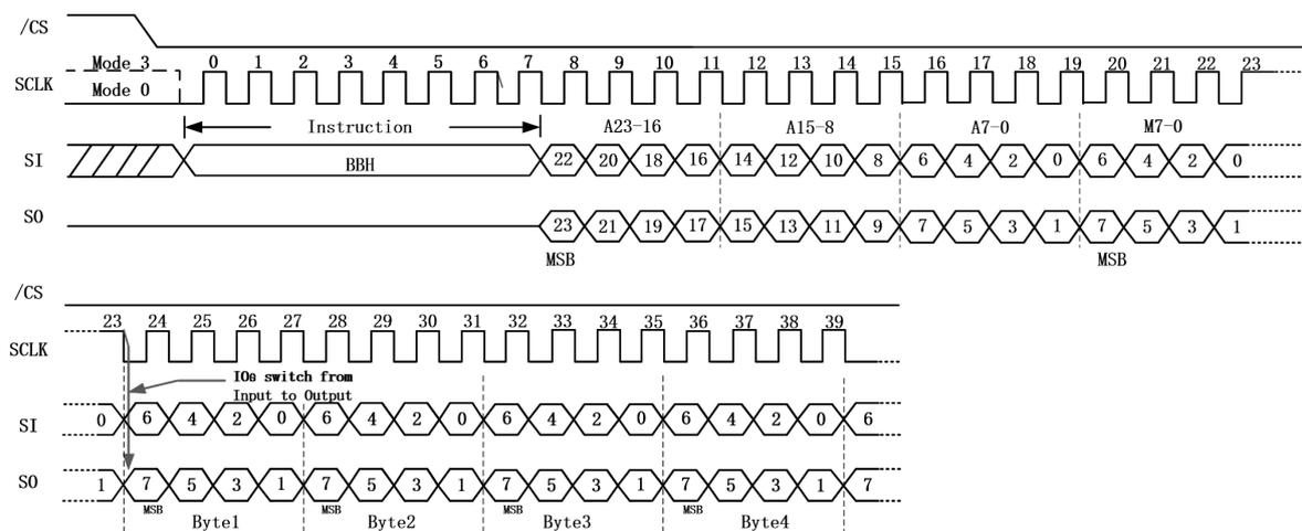
**Figure 7.2.5b.** Fast Read Dual I/O Instruction (Previous instruction set M5-4 = 10)
