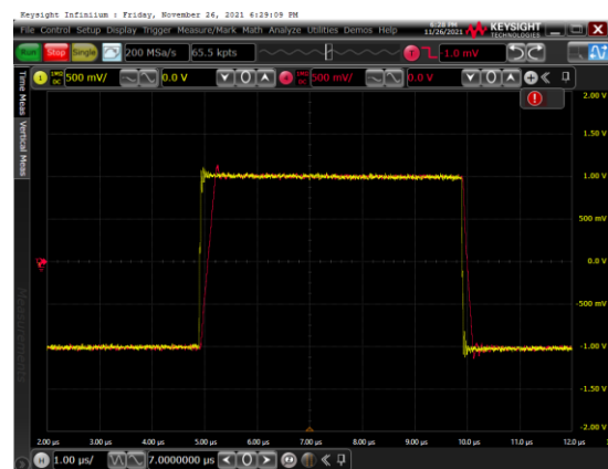
Figure 18 Large Signal Step Response
