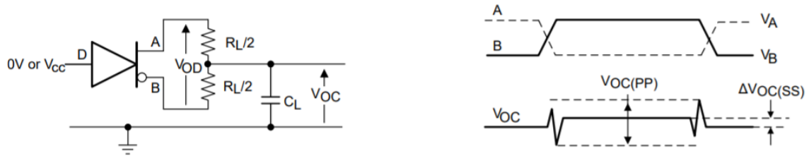
Figure 1. DC Driver Test Circuits
