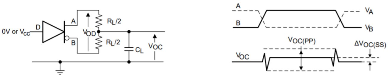
Figure 4. Driver Propagation Delay and Rise/Fall Time Measurement
