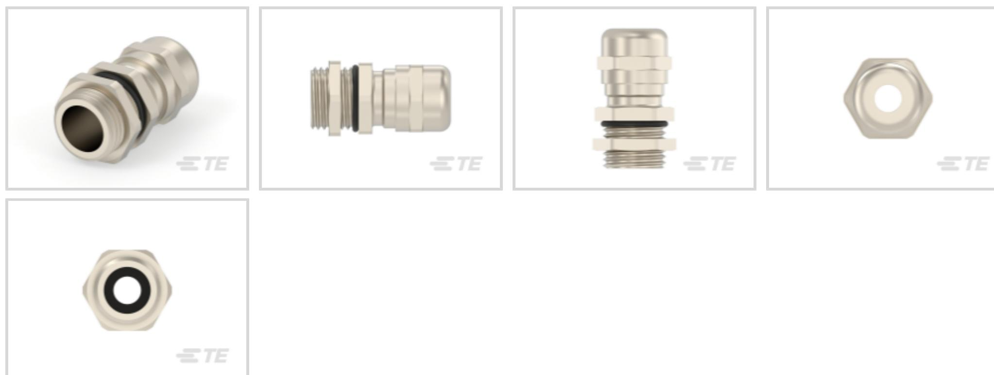
Cable Gland Product Type: **Cable Gland**Cable Gland & Accessory Style: **Standard Threaded**Primary Product Material: **Brass**Clamping Diameter Range: **2. – 6. mm**Primary Product Plating Material: **Nickel**[All Metal Cable Glands With Locknut \(Material Brass\) \(81\)](#)
