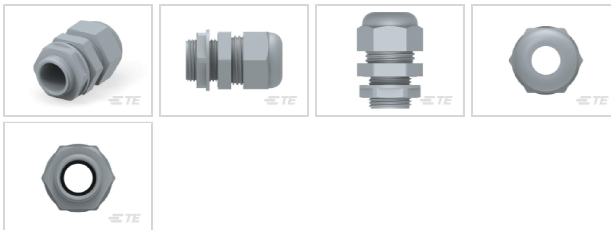
Cable Gland Product Type: **Cable Gland**Cable Gland & Accessory Style: **Standard Threaded**Primary Product Material: **PA6**Clamping Diameter Range: **7. - 12.1 mm**Primary Product Color: **Gray**[All Plastic Cable Glands With Locknut \(177\)](#)
