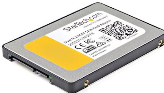
Boost your system performance by enhancing the capacity, speed and security of your data storage. This two-drive M.2 to SATA adapter lets you install two M.2 solid-state drives in a single 2.5" drive bay and configure a powerful RAID array.
