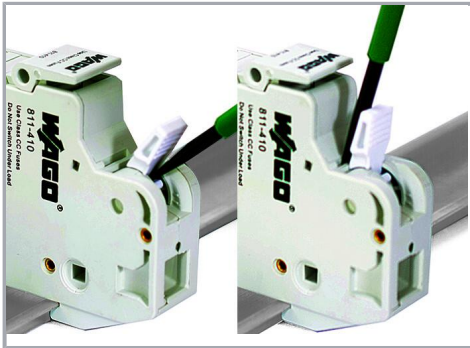
Open and close lever via operating tool.
