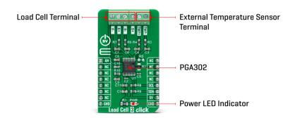
The PGA302 contains two separated analog-front end (AFE) chains with their gain amplifiers for resistive bridge and temperature sensing inputs. The resistive bridge input AFE chain consists of a programmable gain with eight steps from 1.33V/V to 200V/V. For the temperature-sensing input AFE chain, the PGA302 provides a current source that can source up to 1mA for the optional external temperature sensing available on the on-board terminal labeled with TMP+ and TMP-.
