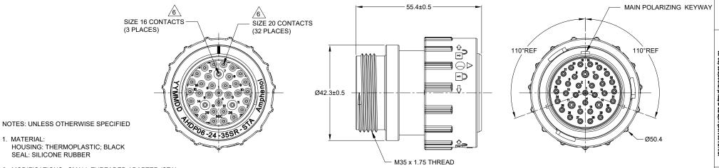
2. MODIFICATIONS: SMALL THREADED ADAPTER (STA); REDUCED DIA. WIRE SEAL;
