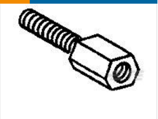
TE Part # 1-829261-6 HD FEMALE SCREWLOCK
