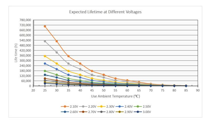
\*Note : Estimated lifespan: The estimated lifespan under different operating voltages and operating temperatures in a theoretical environment. For the actual service life, please contact us to discuss the working conditions.
