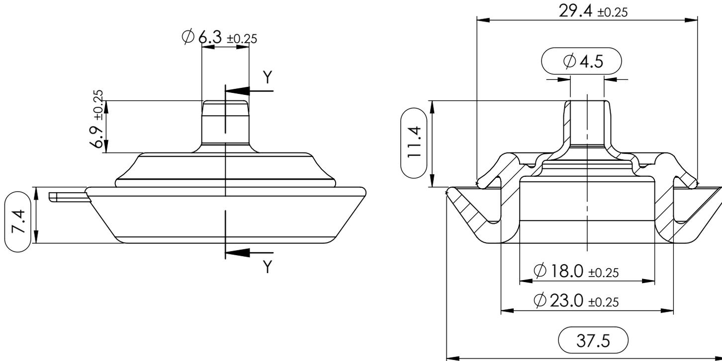
TEST PANEL THICKNESS 1 TO 25
