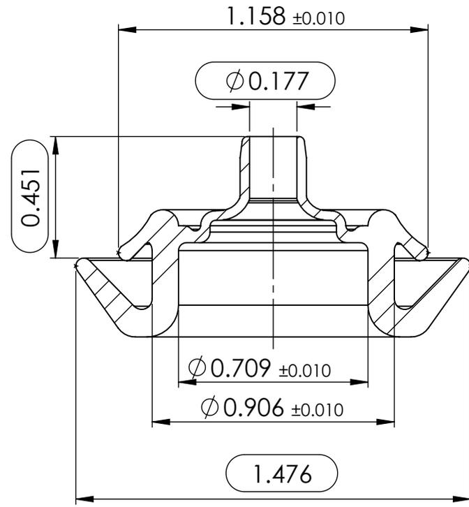
TEST PANEL THICKNESS 0.03 TO 0.984
