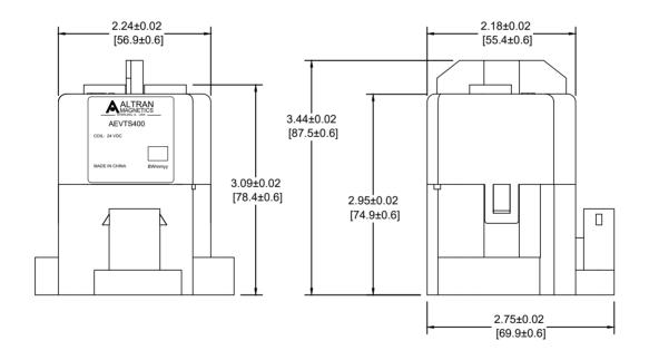
Altran provides Sealed Coil connector for product and hexagon socket screws for contacts, the connector wire length is 180±20mm.
