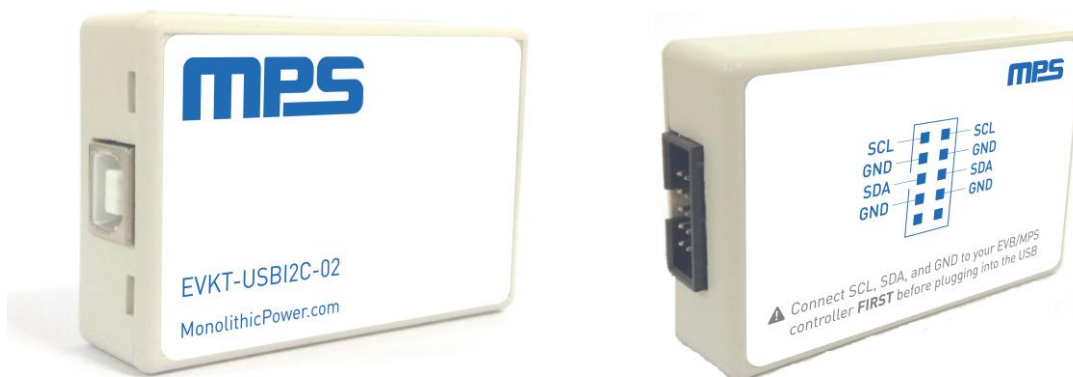
Figure 3: EVKT-USBI2C-02 Communication Interface
