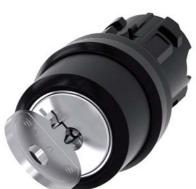
RONIS key-operated switch, 22 mm, round, plastic, lock number SB30, with 2 keys, 2 switch positions O-I, latching, actuating angle 90°, 10:30h/13:30h, key removal O+I, possible special locks: SB31, 421, 455
