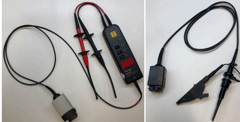
Figure 20: (a) Tektronix® differential probe THDP0200 (1500 V Range), (b) Tektronix TPP0850 voltage probe
