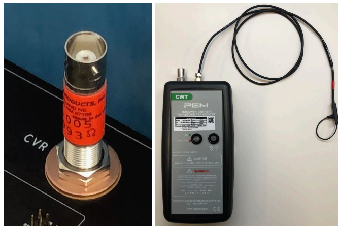
Figure 12: Probe examples, (a) current viewing resistor (T & M Research® SSDN-005, 400 MHz), (b) Rogowski current probe (PEM® CWTUM/3/B, 30 MHz)
