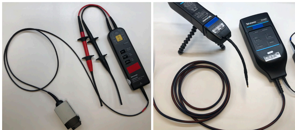
Figure 22: Probe examples, (a) Tektronix® differential probe THDP0200 (150 V Range), (b) Tektronix® IsoVu TIVH05 (TIVPMX10X, ±25 V sensor tip)
