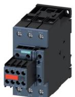
power contactor, AC-3e/AC-3, 80 A, 37 kW / 400 V, 3-pole, 20-33 V AC/DC, 50/60 Hz, with integrated varistor, auxiliary contacts: 2 NO + 2 NC, screw terminal, size: S2, captive auxiliary switch
