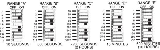
Digital selection of the time delay is accomplished by the use of ten (10) binary switches, each marked with a time increment. The time periods, of which there are five (5) ranges, represented by each switch in the ON position is added together to obtain the desired time delay. No more trial-by-error adjustments.
