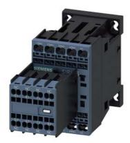
Contactor relay, 4 NO + 4 NC, 110 V AC, 50 / 60 Hz, Size S00, spring-type terminal, Removable auxiliary switch
