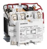
Mechanically held lighting contactor, Contactor amp rating 30A, 0 N.C. / 4 N.O. poles, 110VAC 50HZ/120VAC 60HZ coil, Non-combination type, Enclosure NEMA type (open), No enclosure
