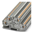
Double-level terminal block, nom. voltage: 800 V, nominal current: 28 A, connection method: Push-in connection, 1st and 2nd level, Rated cross section:  $4 \text{ mm}^2$ , cross section:  $0.2 \text{ mm}^2$  -  $6 \text{ mm}^2$ , mounting type: NS 35/7,5, NS 35/15, color: gray
