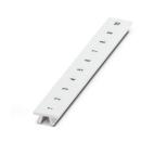
Zack marker strip, Strip, white, labeled, can be labeled with: CMS-P1-PLOTTER, mounting type: snapped, for terminal block width: 8.3 mm, lettering field size:  $10.5 \times 8.3 \text{ mm}$
