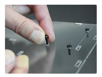
Turn the base over and install three screws in the Arduino footprint area.
