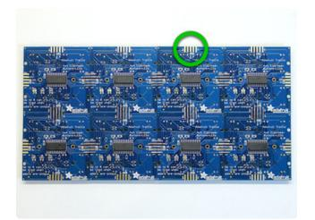
On the HELLA UNTZtrument — a 4x2 assembly of Trellises — connect the wires to the third header along the top edge, not the rightmost fourth header.
