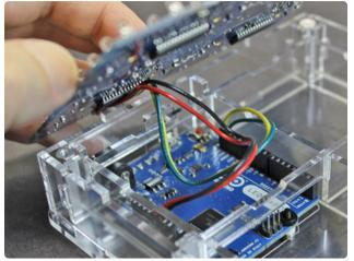
The wires will fight you at this stage, either pushing back against the trellis or springing out of the Arduino sockets. This part goes a little easier if you bend a couple zig-zag kinks in the wires, keeping them all within that quadrant of the case. Be patient and put each wire back in place if they pop out.
