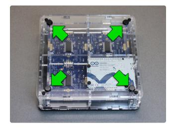
Turn the whole thing over and peel-andstick the four rubber feet near the corners.
