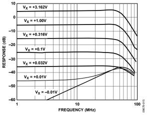
Figure 15. AC Response of the VCA at Different Gains,  $V_{\rm Y} = 0.5$  V RMS
