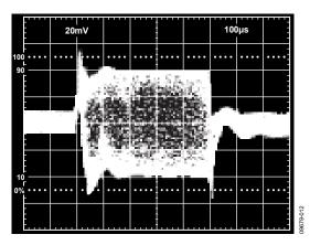
Figure 12. Control Feedthrough One Channel of Figure 22
