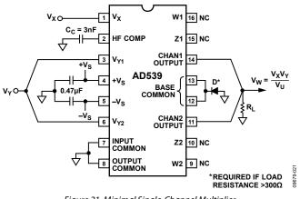
Figure 21. Minimal Single-Channel Multiplier (16-Lead SBDIP and PDIP Shown)
