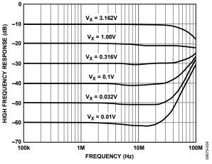
Figure 9. High Frequency Response in Minimal Configuration
