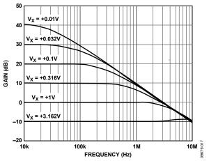
Figure 17. High Frequency Response of Divider in Figure 25
