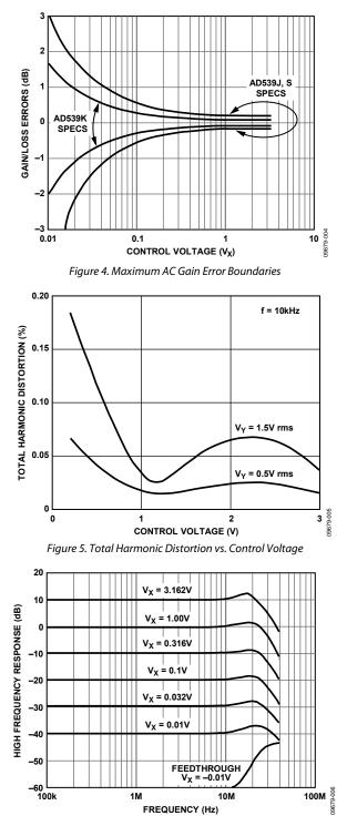
Figure 6. Multiplier High Frequency Response Using LH0032 Op Amps
