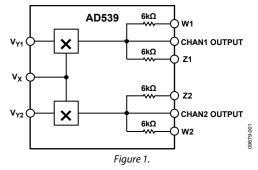
they can be used independently, as in audio stereo applications, with low crosstalk between channels. Voltage-controlled filters and oscillators using the state-variable approach are easily designed, taking advantage of the dual channels and common control. The AD539 can also be configured as a divider with signal bandwidths up to 15 MHz.
