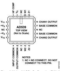
Figure 2. 20-Lead LLC Pin Configuration (E-20-1)
