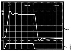
Figure 16. Transient Response of the Voltage-Controlled Amplifier,  $V_X = +2 V, V_Y = \pm 1 V$
