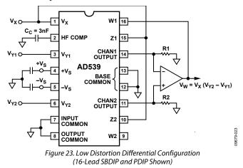
Even lower distortion (0.01%, or -80 dB) has been measured using two output op amps in a configuration similar to that shown in Figure 20 connected as virtual ground current summers (to prevent the modulation effect). Note that to generate the difference output it is merely necessary to connect the output of the Channel 1 op amp to the Z node of Channel 2. In this way, the net input to the Channel 2 op amp is the difference signal, and the low distortion resultant appears as its output.
