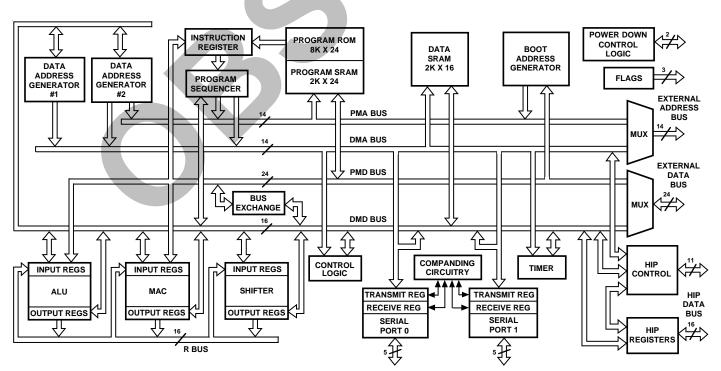
Figure 1. ADSP-217x Block Diagram
