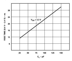
Figure 35. Typical Output Rise Time vs. Load Capacitance,  $C_L$  (at Maximum Ambient Operating Temperature)
