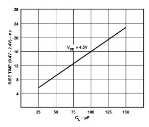
Figure 19. Typical Output Rise Time vs. Load Capacitance,  $C_1$  (at Maximum Ambient Operating Temperature)
